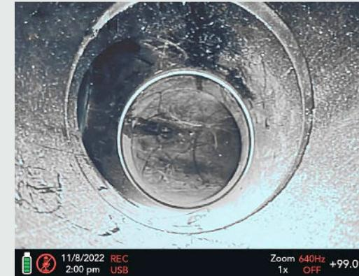
The Hathorn® Info Bar at the bottom of the screen allows you to see battery life, speaker function, time and date, recording file location, zoom, sonde frequency function and footage. The info bar is customizable - allowing you to put your company or client info at the bottom of the screen, recorded throughout the video. The newly designed, intuitive menus allow for a minimal learning curve. You are up and running in minutes.
