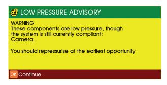
You must press OK to acknowledge this warning. The inspection equipment can still be used as the pressure is still Compliant.
