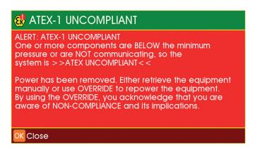
Press OK to acknowledge the alert, and then choose whether to continue using the Uncompliant inspection equipment by switching to OVERRIDE and powering ON again, or whether to abandon the survey and remove the
