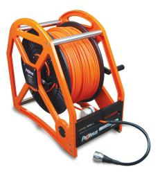
The reels are available in 3 sizes small 100m, mid-size 250m and large 350m reels of high strength, Kevlar reinforced inspection cable with a weight of 5.5kg per 100m and a breaking strength of 500kg. The small and mid-size reels can be fitted to our Portable Storage Trolley (PTP01), and the large reel is ideal for being installed as part of our Custom Van Fit Service.
