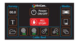
Press *either* key once to cancel continuous paying out or rewinding, and to stop the motor. The motorised cable reel pay out and rewind then goes back to automatic mode.
