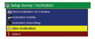
Select "Zero Inclination" and the first stage of the zero calibration begins:
