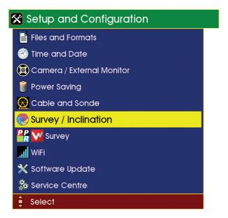
If your crawler supports inclination zero calibration, you will see a menu item "Zero Inclination". If it does not support inclination zero calibration, you can ignore the rest of this setup.
