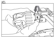
**4** Turn the Locking Ring anticlockwise as shown, to secure the camera in place.
