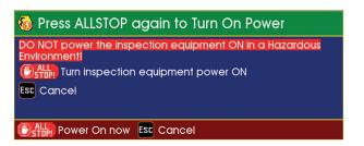
Read and understand any messages shown on-screen, then press the ALLSTOP key to power the inspection equipment ON.
