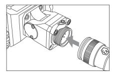
**1** Ensure the cable connector and camera connector are free of dirt, grease and moisture. Offer the cable connector to align with the crawler connector.
