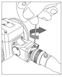
**3** Use a 3mm T-Bar to tighten the Lock Screw, turning in a clockwise direction as shown. **DO NOT** overtighten the Lock Screw.
