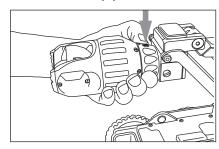
**5** The position of the Locking Grub Screw should now be at the top (12 o'clock).
