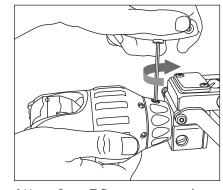
**4** Use a 3mm T-Bar to screw and tighten the Locking Grub Screw. **DO NOT** over-tighten the Locking Grub Screw.
