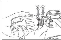
**3** Offer the camera rear connector to the camera connector on the crawler, aligning the Orientation Pin (**D**) on the camera with the Orientation Dot (**A**) on the crawler.
