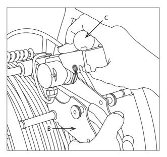
2 Grip the lower arm (B) firmly, and use the knob (C) on the top arm to raise the arm and open the assembly.
