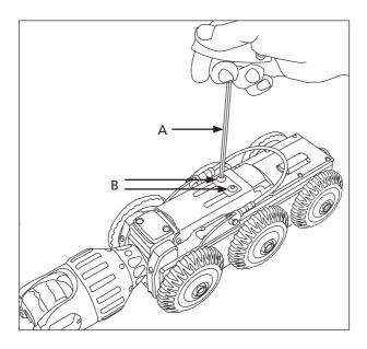
1 Use a 4mm Allen Key (A) to loosen the two hex bolts (B).
