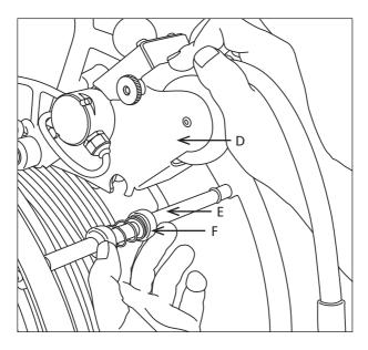
3 To release the assembly (D) from the meter counter bar (E) squeeze the spring clips (F) while lifting the assembly.
