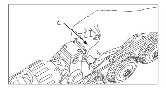
2 Grip the elevator arm (C) firmly and pull upwards to the required height position. Secure the elevator using the 4mm Allen Key to tighten the hex bolts.
