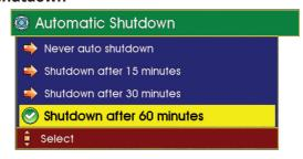
When the SOLOPro+ is powered only by internal batteries this feature will power down the SOLOPro+ after a period of inactivity.
