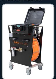
The Sewertronics' QuickPatch LED cures prepregs for a spot repair from 4-18". QuickPatch's high-power LED design incorporates a breakthrough, shadowless technology that guarantees full radiation reach to the entire surface of the Fiberglas prepregs. Each QuickPatch UV LED packer features a axial view camera for precise positioning and monitoring during curing.
